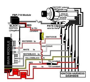
Connecting the FBP-718 to the RS-1100 SERIES units with On-Board Relays.
